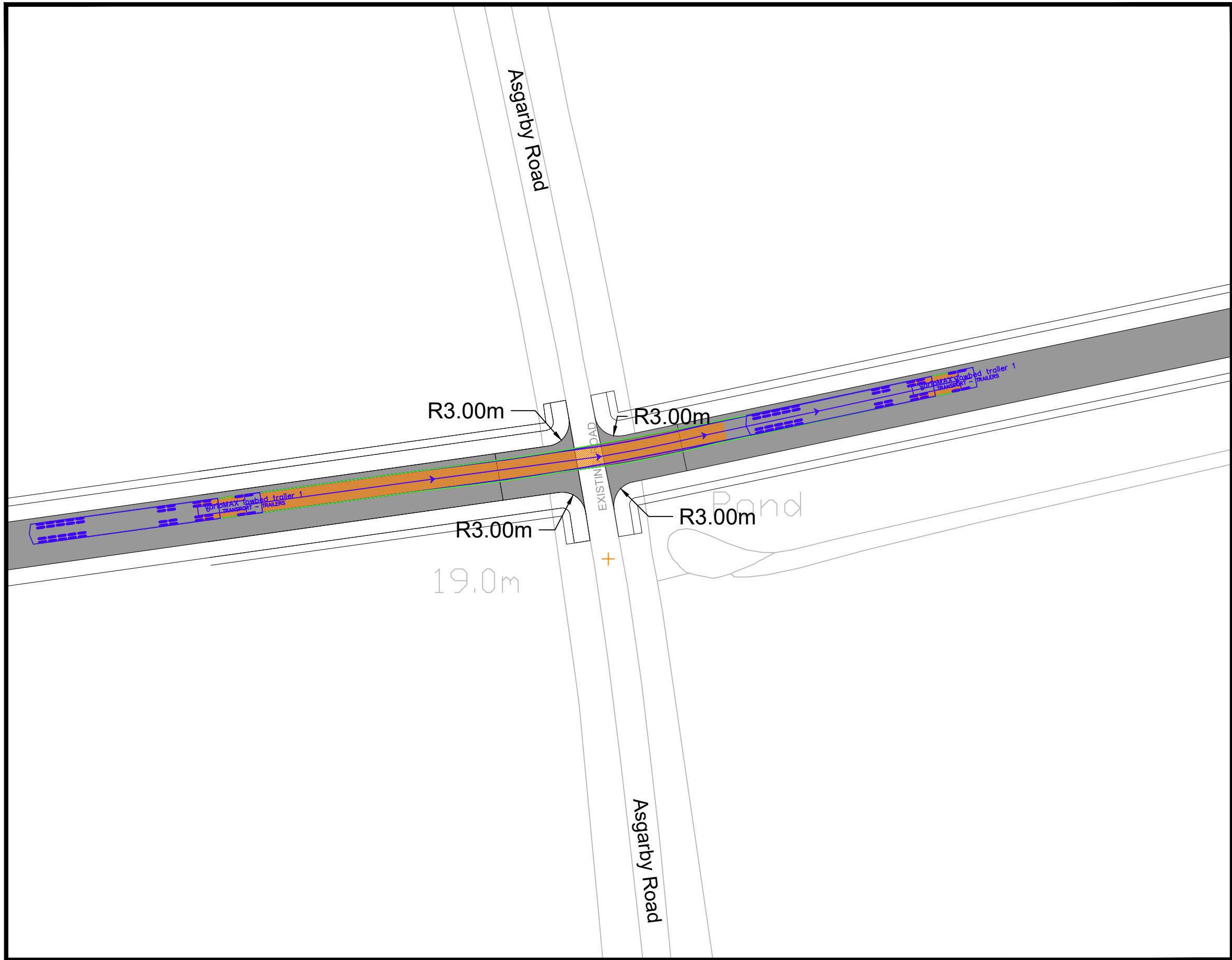
SWEPT PATH ANALYSIS: LOWBED TRAILER- 27.63M SCALE: 1:500
